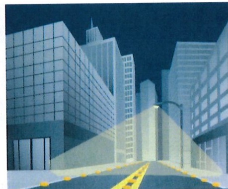
The dotted lines in the graphic above represent our method – which collects light measurements from significantly more locations – providing a comprehensive understanding of the fixture's light distribution pattern and photopic/scotopic performance.
